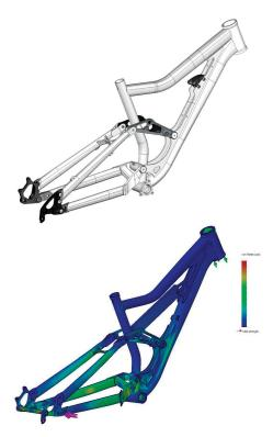
With SolidWorks Motion and SolidWorks Simulation software, Cycles Devinci engineers use a virtual test bench to simulate frame performance and optimize strength-to-weight ratios.
