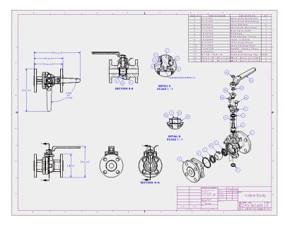
2D drawing views are automatically created from the 3D model and updated whenever the model is changed.
