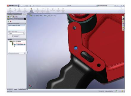
SolidWorks software checks hole alignment automatically.
