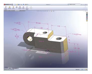
With SolidWorks software you can automatically dimension 3D models according to industry standards.
