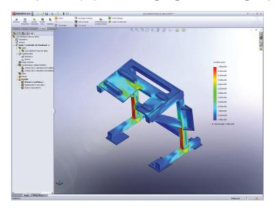
SolidWorks software provides an array of simulation and optimization tools to help you calculate forces due to motion, part stress, and deflection as well as vibration, flow, and effects of temperature.
