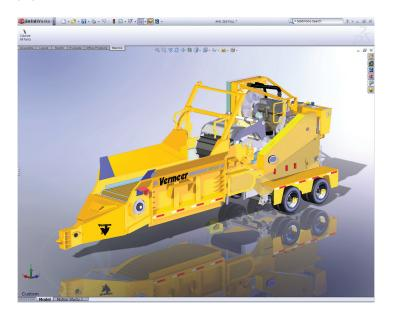
Vermeer uses SolidWorks software to check for interferences and collisions in large assembly designs, which range from 500 to 4,000 parts.
